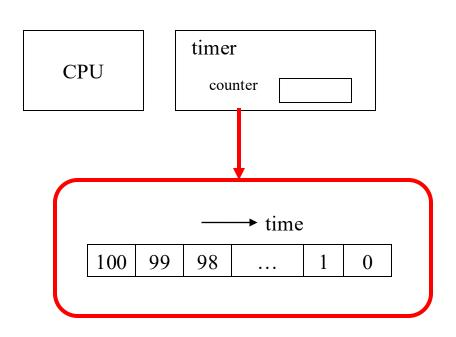
The timer sends an interrupt to CPU when time-up
